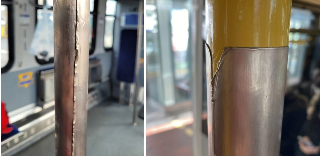
Figure 11: Copper decal vandalism
